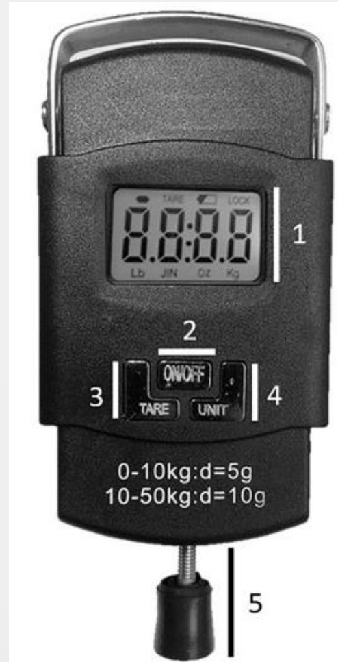
Figure 1 Adapted pressure algometer—PA. (1) Display; (2) On-Off button; (3) Tare button; (4) Unit selection button; (5) Adapted terminal. Full-size DOI: 10.7717/peerj.10162/fig-1
