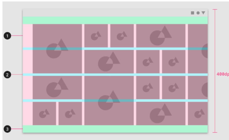
Figura 21 – Grid Horizontal: (1) Coluna (2) Gutters (3) Margens
