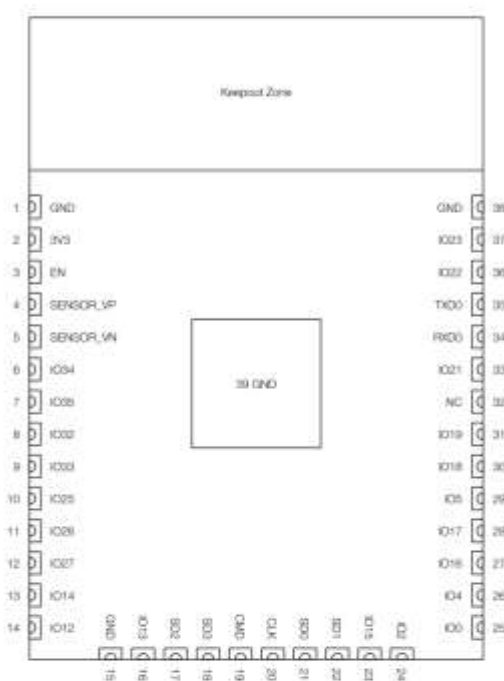
Figure 1: ESP32-WROOM-32 Pin Layout (Top View)
